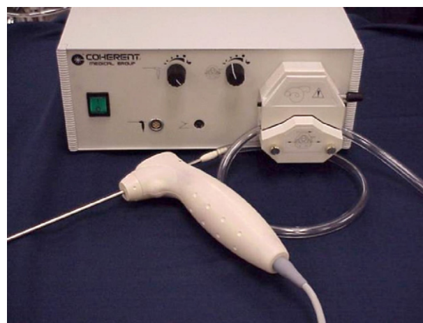
Fig. 2 – The mechanical morcellator uses reciprocating blades, an ergonomic hand piece, and a two-stage foot pedal attached to a controller box that contains a high-powered suction pump.
